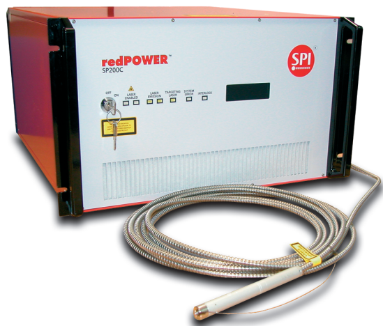
High powered 1090nm water cooled fiber lasers, 100W to 200W, TEM 00 (M 2 <1.1) CW or Modulated to 10kHz closed loop, 50kHz open loop - Modulated pulses 10µs to CW
