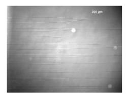
Figure 4: Phase contrast micrograph of a series of 1x2 splitters femtosecond laser inscribed in silica. Arrays such as these are used to characterise losses and identify optimal designs.
